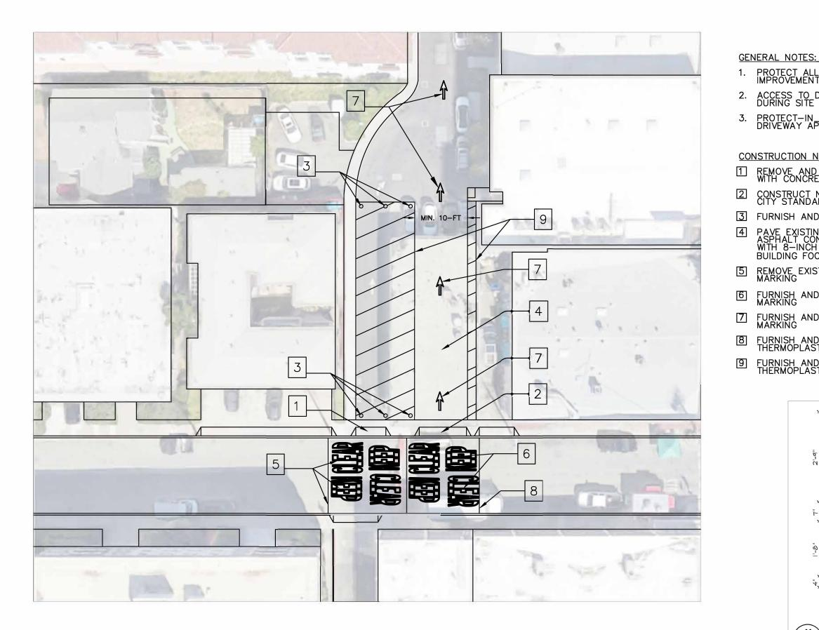
PROTECT ALL EXISTING BUILDINGS, STRUCTURES, AND IMPROVEMENTS OUTSIDE OF THE PROJECT SITE. ACCESS TO DRIVEWAYS AND BUSINESSES SHALL REMAIN DURING SITE DEMOLITION AND RESTORATION. PROTECT-IN\_PLACE SIDEWALK, CURB, GUTTER, AND DRIVEWAY APPROACHES UNLESS OTHERWISE NOTED.
